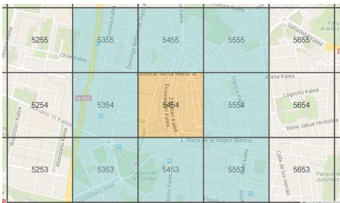
The 'huellasolar databuilder' checks if there are files of data of the tiles adjacent. This way they are taking into account in the calculations of shadows and the reliability of the data when we are near the bounds of the tiles is better.
